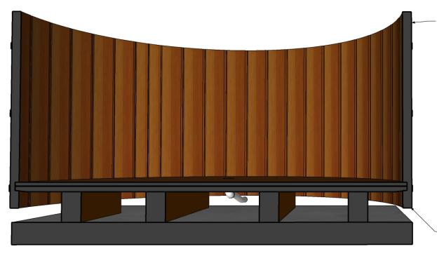
No lateral (sideways) forces against the staves. Do not over tighten the upper most staves. The staves must remain straight vertical.
