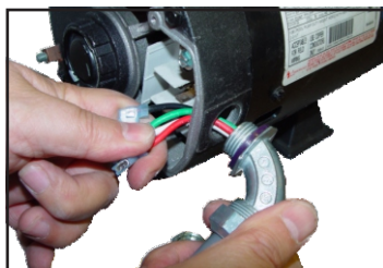
3) Route the power wires through the conduit hole and pull toward you to allow for the cord assy to be rotated for tightening.
