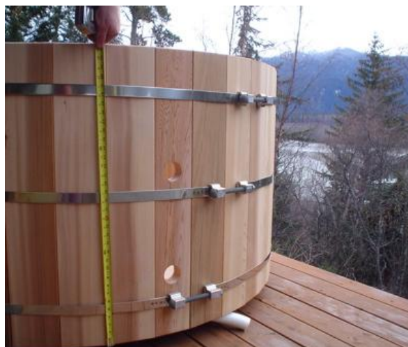
Proper placements of bands and bolts. Note how the bolts straddle seams and are staggered.
