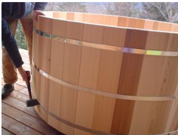
Figure 8.1 Hitting staves directly on the band.
