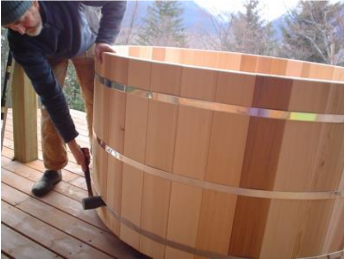
Figure 8.1 Hitting staves directly on the strap.
