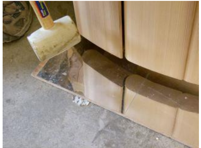
Figure 6.1.1 Mirror allows you to see the bottom of the staves. USE IT!
