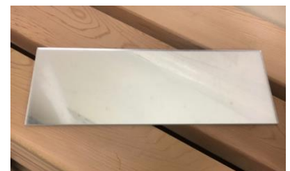
Mirror for seeing bottom of staves during assembly
