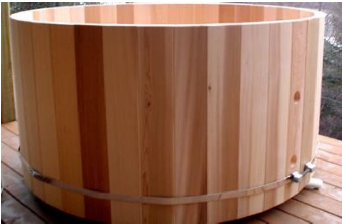
Figure 7.1 first compression strap loosely in place.
